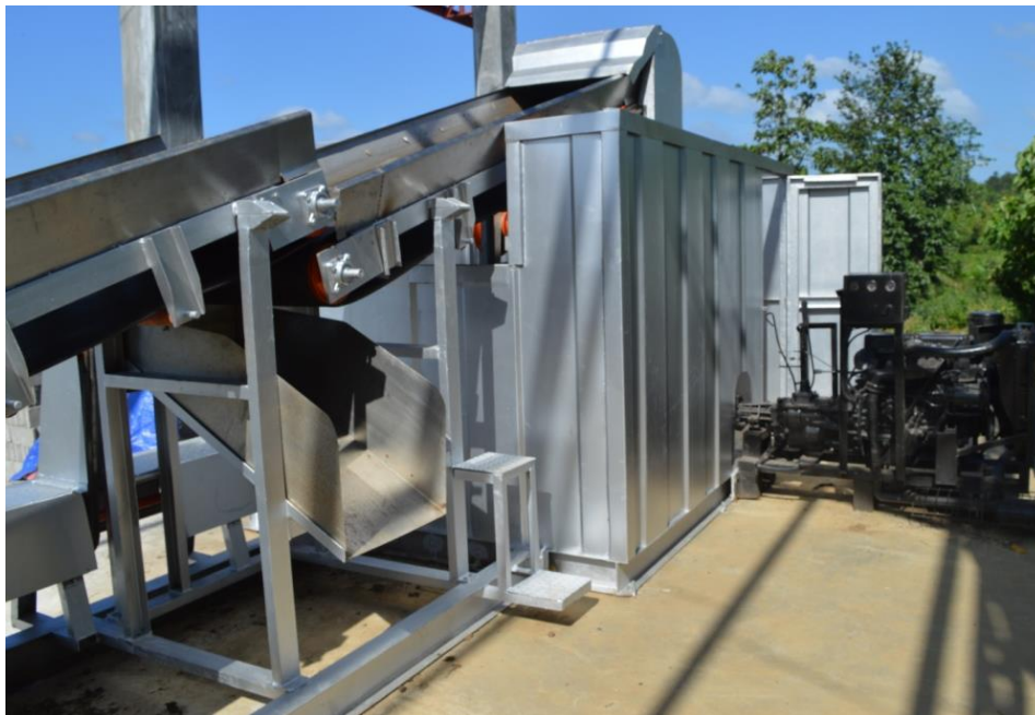
Granulator's Diesel Engine 4D30
